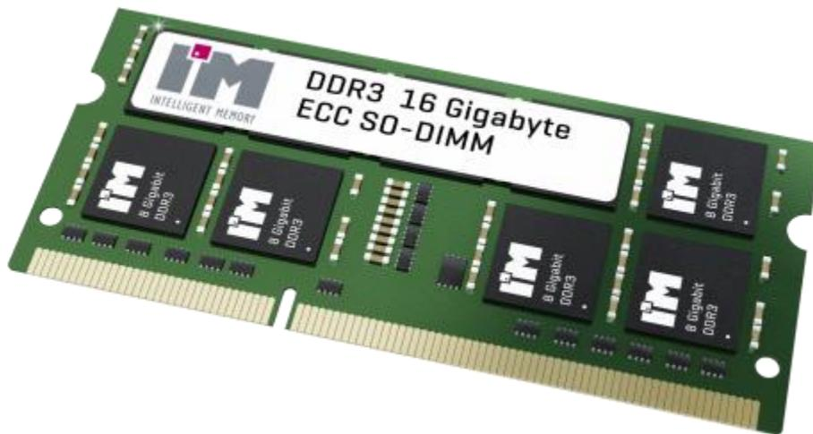
**Figure 3.** *This 16GB DDR3 SO-DIMM allowed the AXIe digitizer to double available memory to 128GB, enabling 3 second gapless recording times at 40GS/s. The power and cooling capability of AXIe allows dense high speed memory directly onto the module, bypassing any speed limitations of an external bus.*
