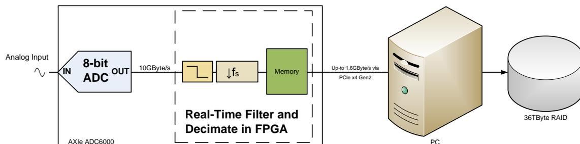
**Figure 1.** After the signal is digitized and (optionally) processed and managed in memory, it is streamed to the PC controller via PCI Express. On-board the PC, it is streamed to another PCI Express port where a RAID array of 36TByte or more may be storing the gapless data.
