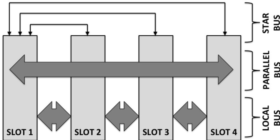
**Figure 2.** Parallel buses such as trigger buses traverse all slots, and serial buses such as PCI Express are arranged in a star configuration to each slot. Local buses, however, connect only between adjacent slots. The short length enables very high data rates.
