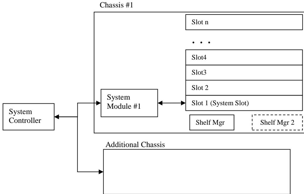
**Figure 1 Hardware Components of an AXIe System**
