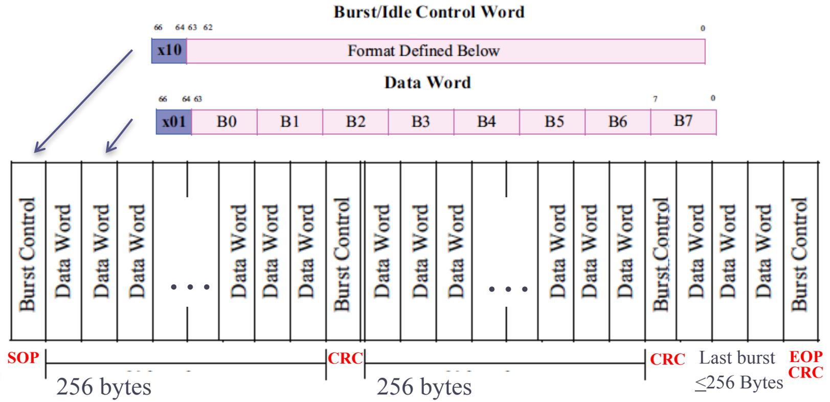
Start of Packet and End of Packet encapsulate one packet.
