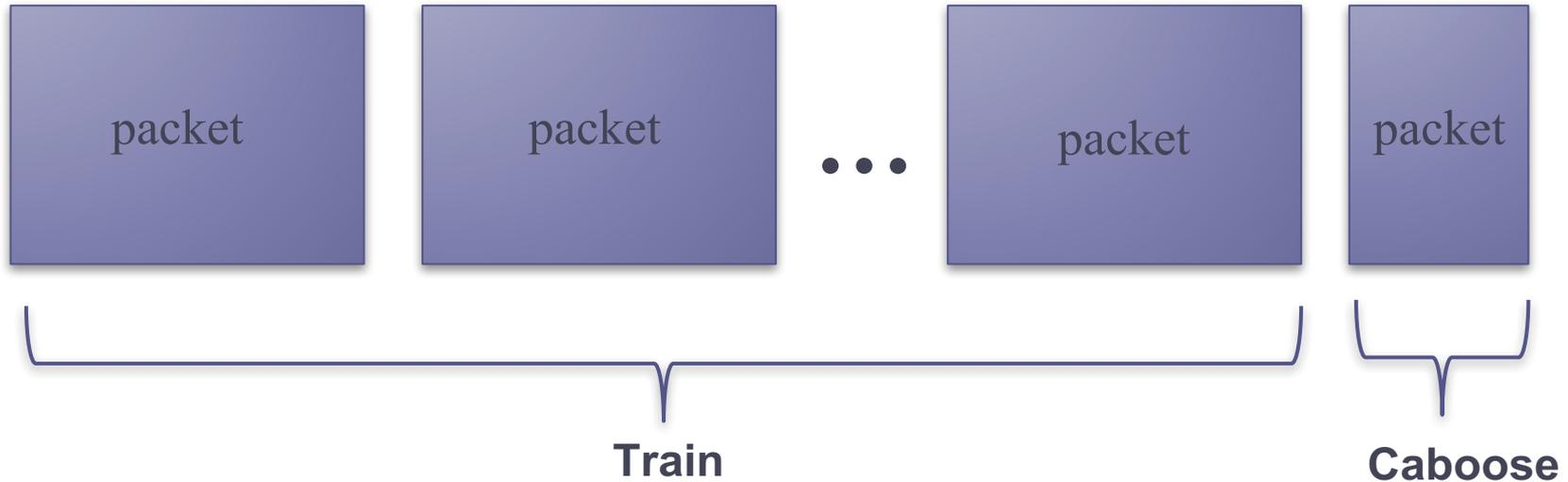
Streaming is performed by transmitting a series of large packets consecutively in a “train”. These packets are designed for efficiency, and typically are of the same length and number of samples.
