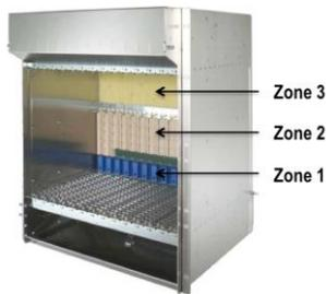
AXIe also includes an optional customizable backplane area known as Zone 3. Essentially it is an empty space where a custom backplane may be inserted, or signals can be routed. Since standard AXIe-1 modules don't access Zone 3, they may be inserted into a chassis that does so, without conflict. These features together make AXIe an attractive platform for system integrators.
