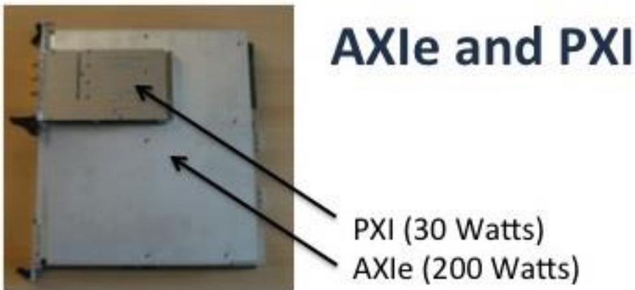
**The image above highlights the difference in modules size between AXIe and PXI.**
