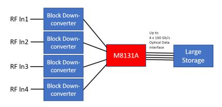
captured simultaneously using a single M8131A module. Combined with a compatible block down-converter, frequencies up to 44 GHz with modulation bandwidths up to 4 GHz can be captured.
