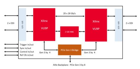
the module provides a trigger input and output, synchronization input and outputs for deterministic latency between compatible digitizers and AWG modules as well as a 10-general purpose I/Os.
