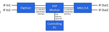
one or more digital signal processing modules can be inserted in the path.
