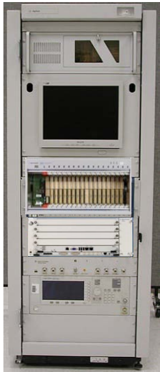
LXI, PXI, and AXIe Rack and Stack System
