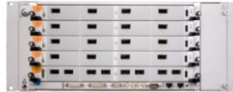
5-slot 4U integrated chassis
