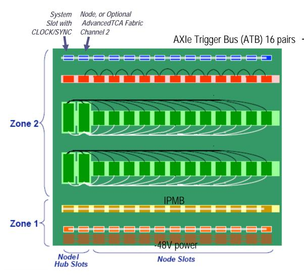
ToomHz CLOCK, 1 pair point-to-point SYNC, 1 pair point-to-point STRIG, 1 pair bi-directional point-to-point Triggers, 13 pairs MLVDS
