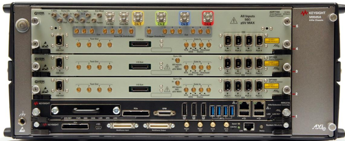
Figure 1 shows the first ODI products to be announced. The Guzik ADP7104 AXIe digitizer, on top, has four ODI ports shown in the lower right corner of the module. The product can stream two channels, each at 10-bits and 32Gsamples/s, continuously to the DP7000 digital processing modules shown
